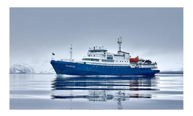
M/v *Plancius* was built in 1976 as an oceanographic research vessel for the Royal Dutch Navy and was named "Hr. Ms. *Tydeman*". The vessel was completely rebuilt as a passenger vessel in 2009 and complies with the latest SOLAS-regulations (Safety Of Life At Sea). M/v *Plancius* is 89 m long, 14.5 m wide and has a maximum draft of 5 m, ice class 1D, 10,5 knots average cruising speed and has 3 Diesel- Electric engines.
